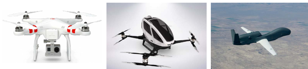
Figure 1.1 Examples of drones: DJI Phantom (Class 1, left), Ehang 184 (Class 2, centre), Northrop Grumman Global Hawk (Class 3, right). Source: DJI, Ehang and Northrop Grumman.
