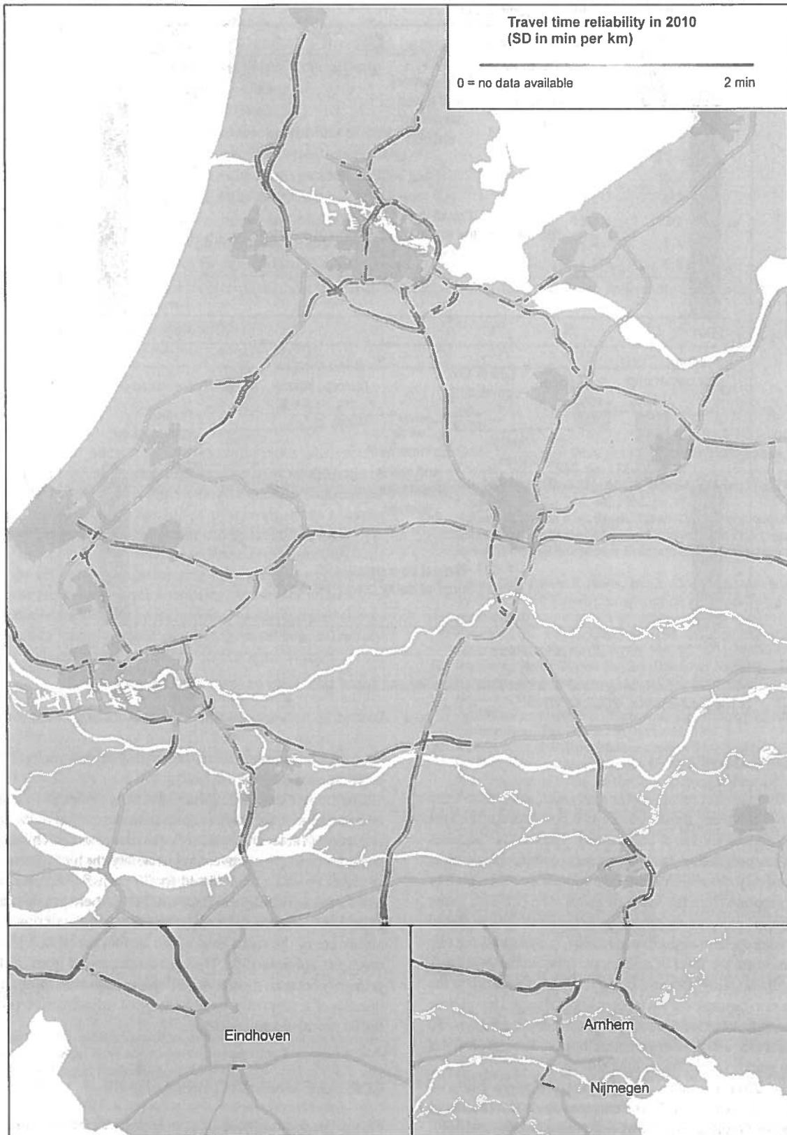
FIGURE 6 Spatial differences in travel time reliability in relation to SD on main trunk network in the Netherlands.
